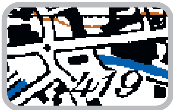
In a 10 times enlargement of the pixel map, the original pixels are rather coarse (0.5 mm)
