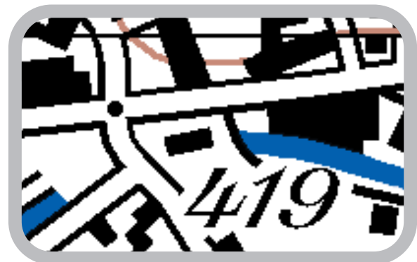
In a 10 times enlargement of the vector map, the standard screen resolution (0.3 mm) is maintained
